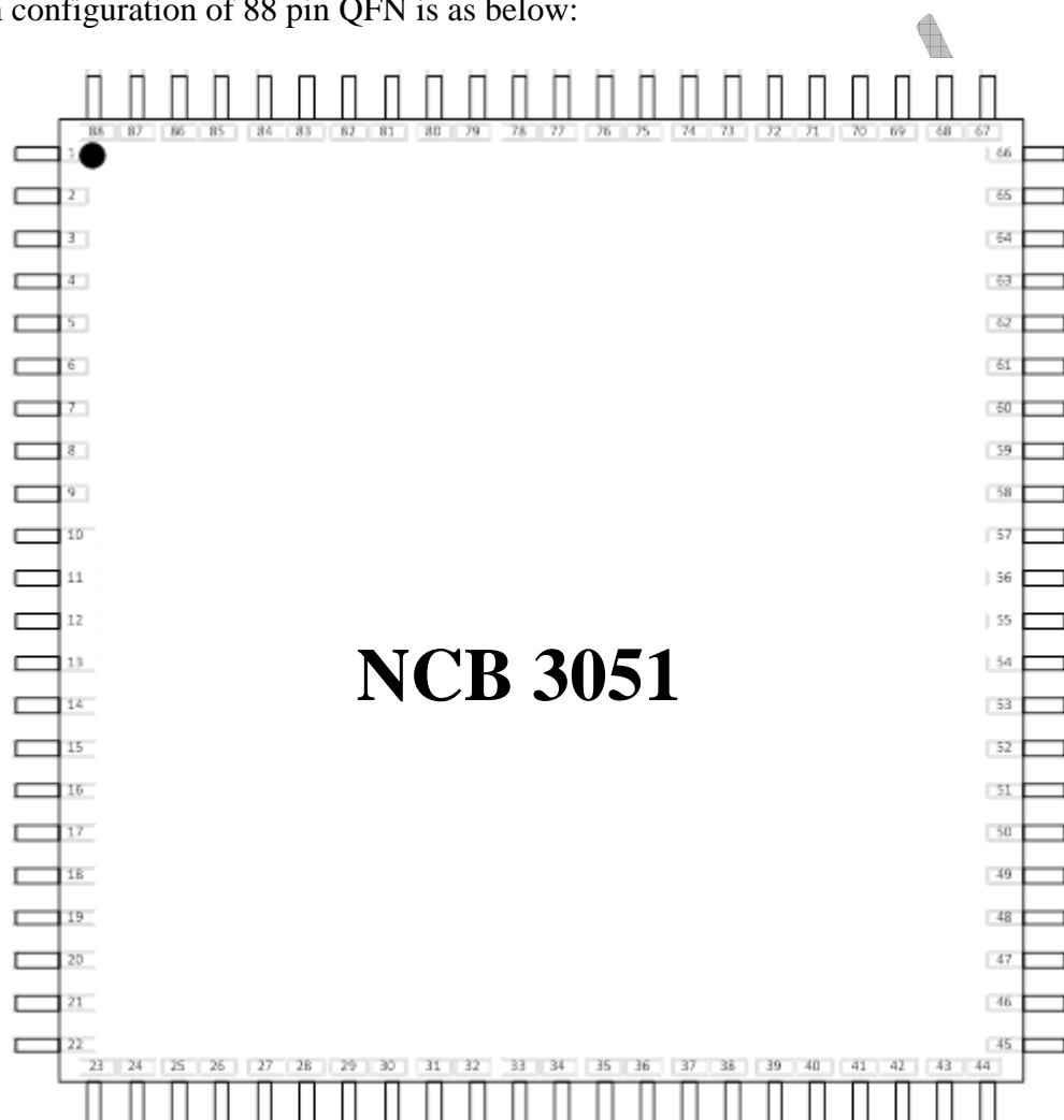
Figure 0-1 Package pin configuration (QFN88)
